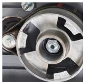
Simple to Maintain & Service Tensioned belt and pulley mechanism - no complex cogs/ gear wheels
