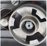
**Tried & Tested Drive System** pulley Tensioned belt and mechanism - no complex cogs/ gear wheels
