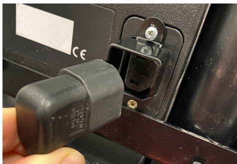
Attach the power cable
